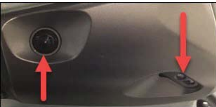
Figure 98: Right side 2D and 3D cameras
