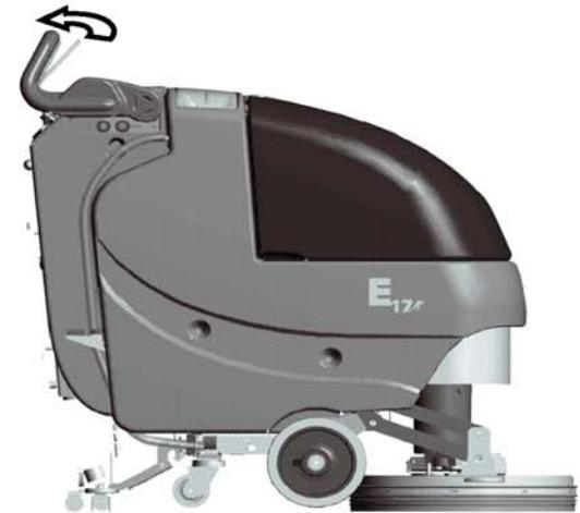
3. With the key turned on, pull the bail handle to engage the scrub brush onto the scrub deck.
