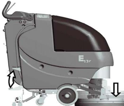
2. Lower the scrub deck by releasing the deck lift pedal.
