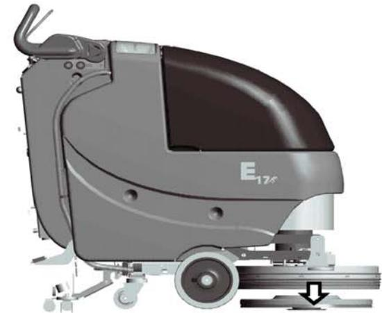
3. When done correctly the brush should release from the scrub deck and fall to the floor.
